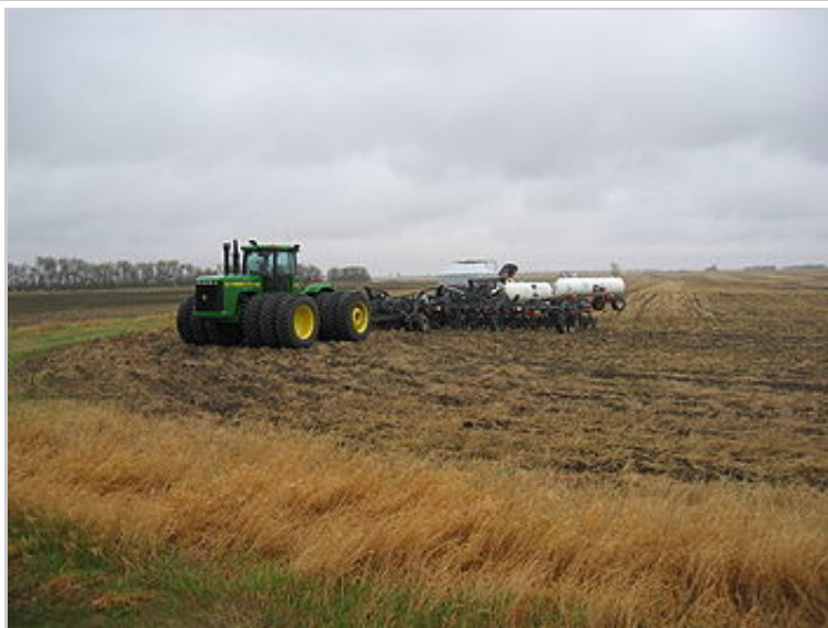
A large, modern John Deere model 9400 four-wheel drive tractor with triple wheels and a drawbar-towed tool chain, including one-pass tillage equipment, planter and fertilizer applicator with tanks
