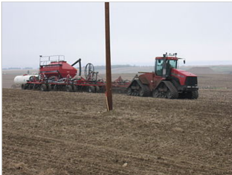
A modern steerable all-tracked power unit planting wheat in North Dakota
