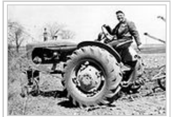
The classic row crop tractor (an Allis-Chalmers WD) - note the absence of any rollover protection system.
