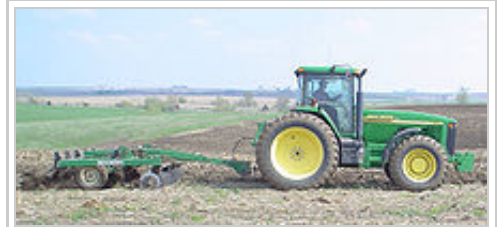
A modern John Deere 8110 Farm Tractor using a chisel plough. The ploughing tines are at the rear; the refuse-cutting coulters at the front.
