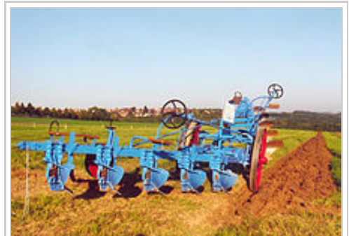
A German balance plough. The left-turning set of shares have just completed a pass, and the right-turning shares are about to enter the ground to return across the field.
