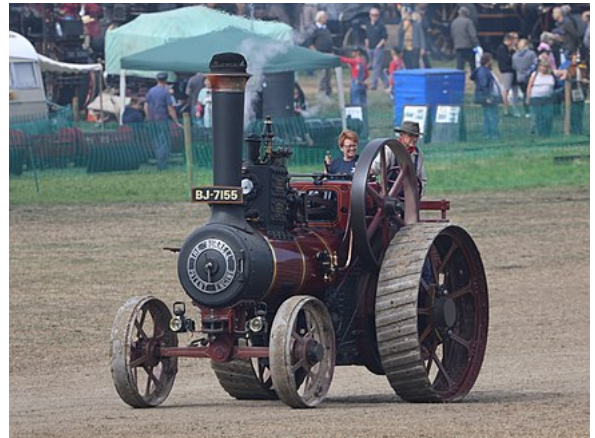
A typical preserved traction engine: 1909 Burrell 6 nhp general purpose engine, at Great Dorset Steam Fair in 2018.
