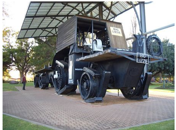
"Big Lizzie", a purpose built tractor with two trailers, designed and built by Frank Bottrill using the Dreadnaught wheel which he designed. When built "Big Lizzie" was the biggest tractor in Australia and thought to be the biggest in the world, at 34 feet high by 18 feet wide, and weighing 45 tons.
