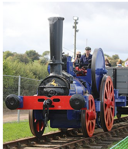
An Aveling and Porter traction engine-based railway locomotive, as used by Holborough cement co.
