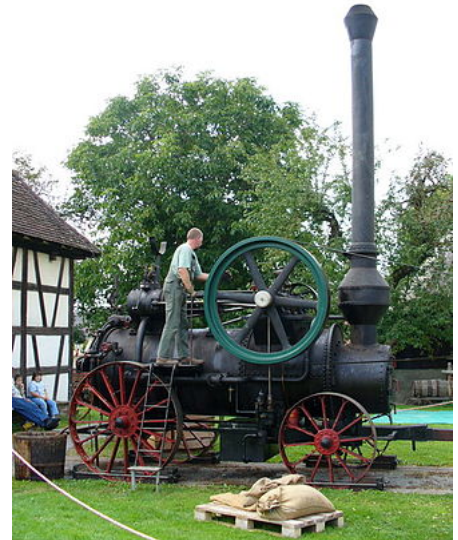
Portable engine showing the lack of self-driven wheels
