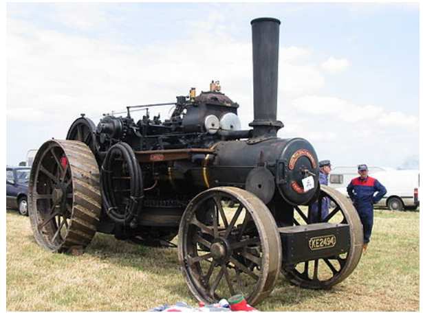
A John Fowler & Co. Ploughing Engine - the winding drum is mounted below the boiler (the 'drum' on the side is actually a hose for refilling the water tank). A lockable tool box may be seen on the front axle; the 'spud tray' would be mounted in the same way, behind the axle.
