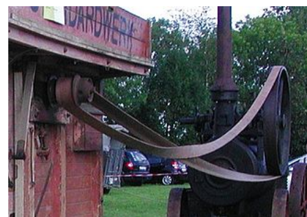
The drive belt: used to transfer power from a portable engine to a threshing machine
